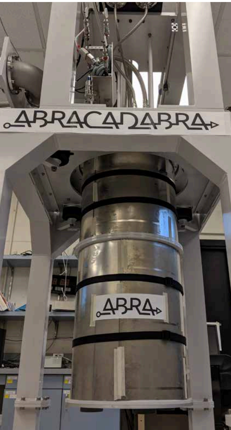
FIGURE 1 The ABRACADABRA-10cm experiment installed and ready to take data in its dilution refrigerator in MIT's Building 24.
